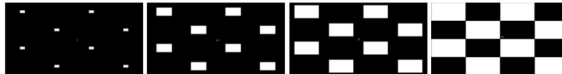
Figure 2: ANSI-like patterns with varying levels of white field representation (APL) between 1% and 50%.
